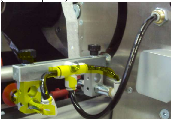
N100811 Vacuum cup with holder and tubes to match with double cup (marked parts)
