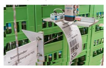
The system consists of a high-quality label printer from NOVEXX Solutions with knife, USI interface and additional display. This robust label printer is very suitable for the application, especially due to the print head and the film saving function. Labels in A5 format are printed with it and securely attached to the twine with special pliers directly during strapping.
